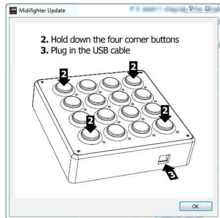
As before hold the four corner buttons for 5 seconds after reconnecting the USB cable, or until you see the checker board pattern.
